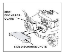
Only Mulching: the chute should be removed and the discharge guard flap closed.
