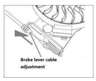
Engine brake adjustment:
